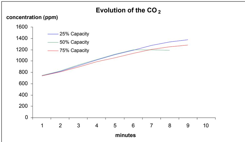
Pic. 3. CO<sub>2</sub> rate evolution with equipment turned on during combustion.
