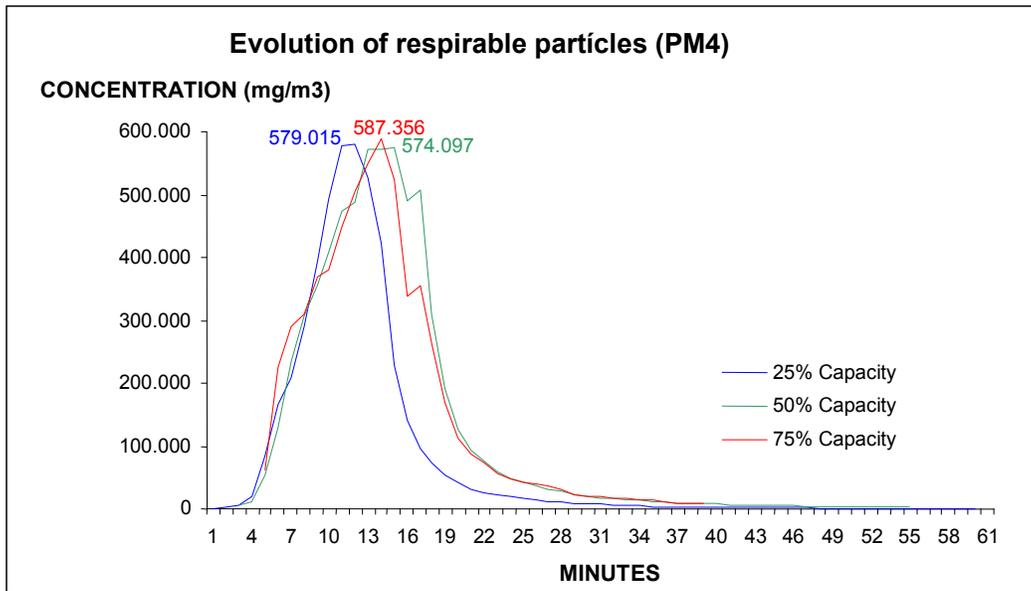
*Pic. 2. Evolution of RSP with equipment off during combustion*
