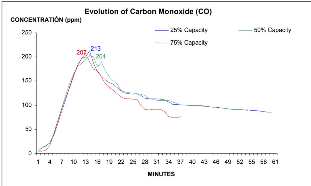
Gráf. 6. CO rate evolution with equipment turned off during combustion
