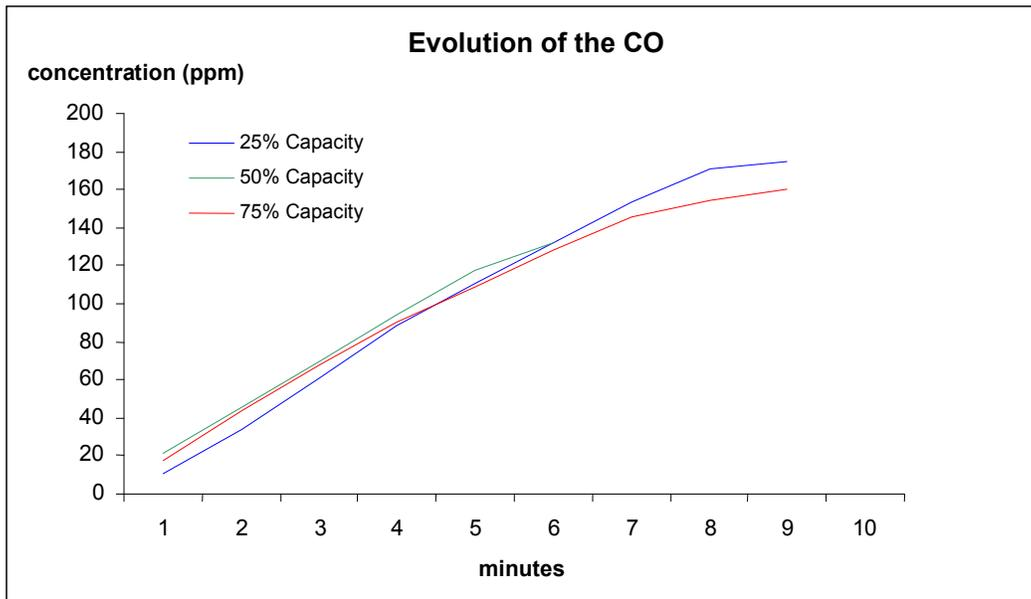
Gráf. 5 CO rate evolution with equipment turned on during combustion
