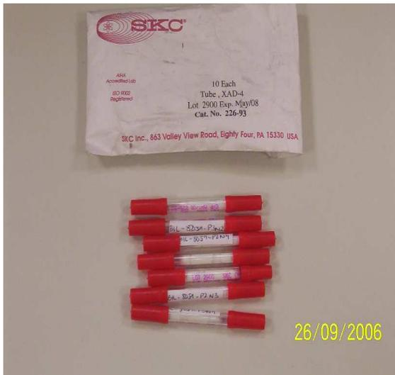
Fig 4. XAD-4 adsorbents, 80/40 mg
